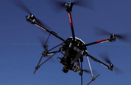
The calculation of the exact volume of stockpiles, rock piles or quarries has never been so easy, quick and exact. Our XR6 stockpile system flies fully automatically and records the dimension from the air with millions of image measurement points in a few minutes.
