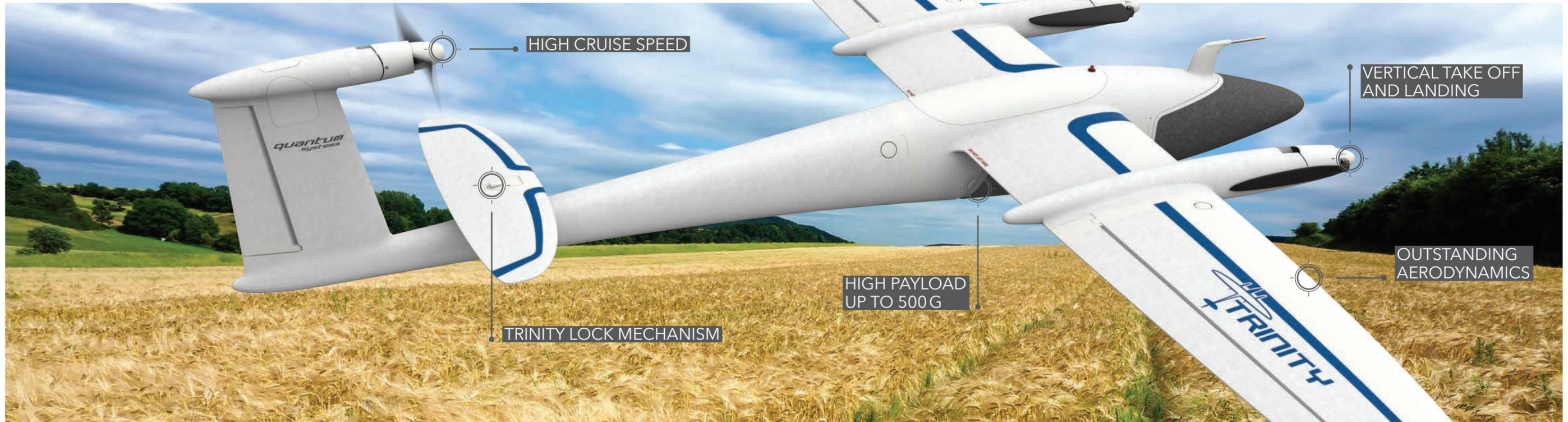
The TRINITY combines high efficiency, flexible mission capabilities, and a small, portable footprint. The result is the world's most compact VTOL fixed-wing drone available today!
