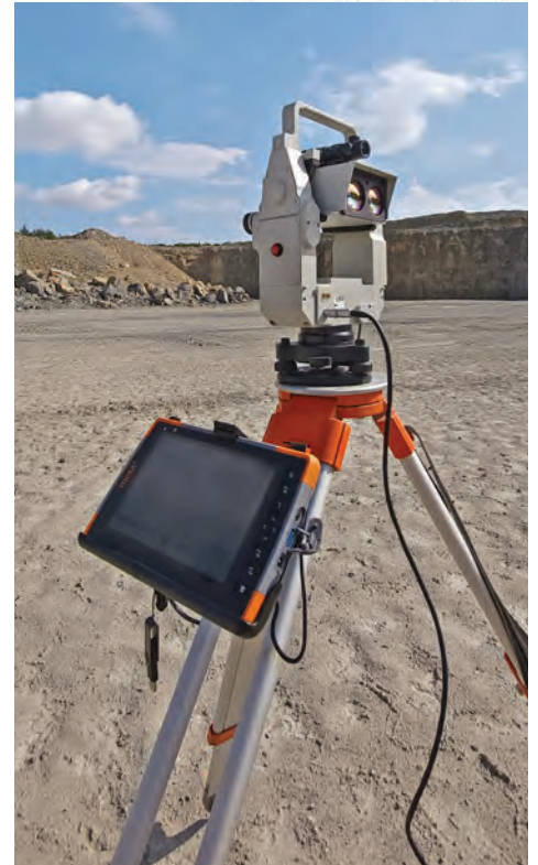
The Mesa Rugged Tablet displays data from geo-konzept's QuarryX software as the borehole positions are planned in the quarry.
